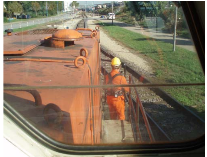
Shunting duty: remote control of the tractive unit from the auxiliary driving position
