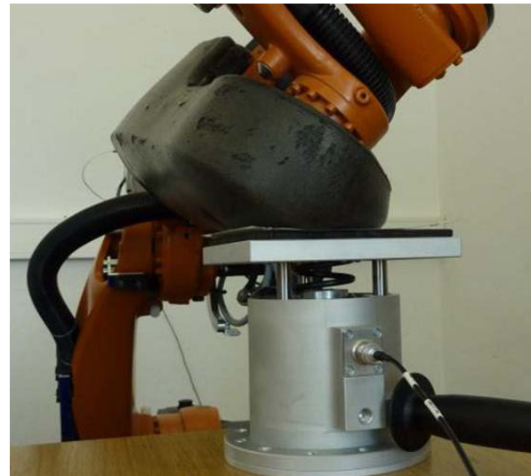
Robot applying force to the measuring instrument (Source: MRK-Systeme GmbH)
