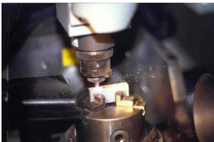
Figure 6: Surface machining of ceramics
