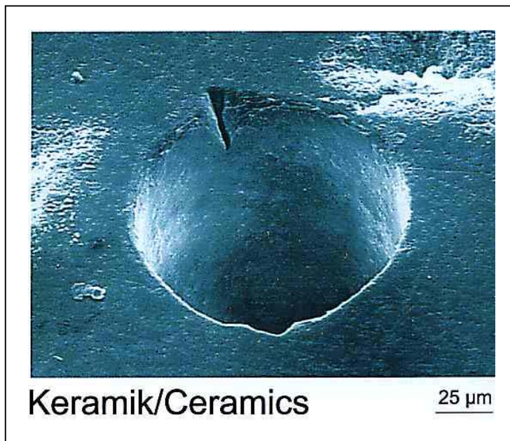
Figure 5: Precision machining of ceramics using copper vapour lasers
