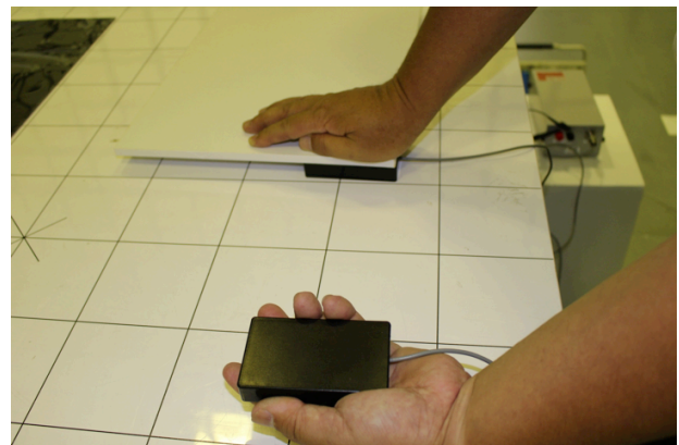
Figure 7: Setup of quasi-contactless communication via human body
