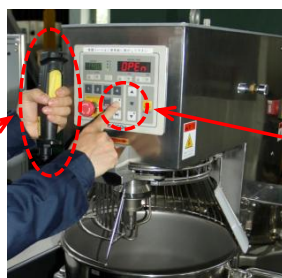
Figure 6: Food processing mixer (with 3 position enabling device + hold-to-run control device)
