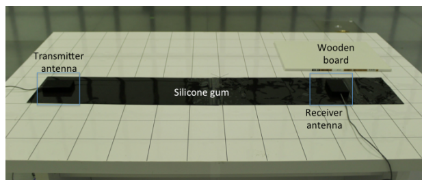
Figure 5: Setup of contact communication via mimic skin
