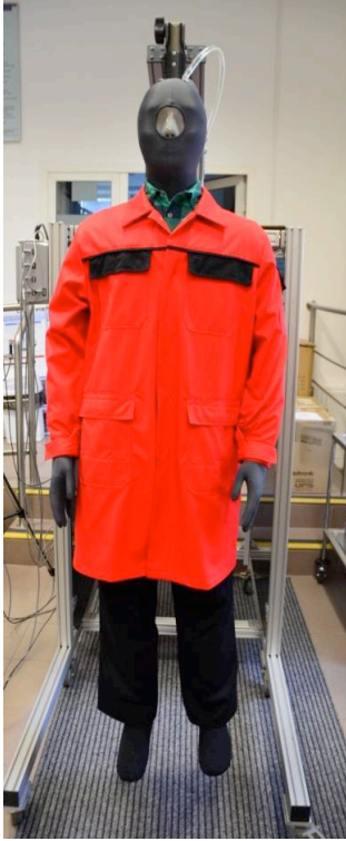
Fig. 18. Picture of manikin dressed in in prototype of the system for measuring undergarment temperature and relative humidity with data logging and wireless data transmission
