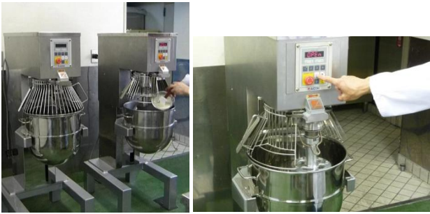
Figure 5: Food processing mixer (with interlock mechanism, hold-to-run control device)
