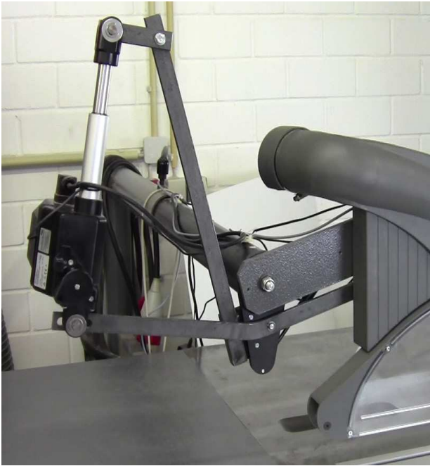
Figure 3: Electrical lifting cylinder and transmission setup
